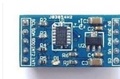
Gambar 2.5 Accelerometer ADXL345 Triple Axis
