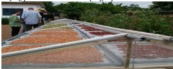
Figure 2. Drying using a solar tunnel dryer
